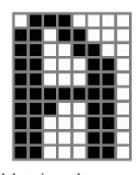
To allow for graphic block, all bits of each byte are used. In the default font B0 of each byte is used as space.
